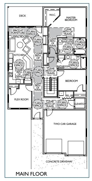
Figure 2: Accessible paths of travel in a residence Diagram by Ron Wickman, Architect
