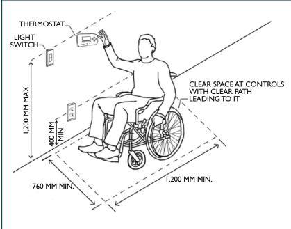
Figure 9: Optimal reach range for controls Diagram by Ron Wickman, Architect
