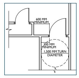
Figure 4: Clear floor space at doors Diagram by Ron Wickman, Architect
