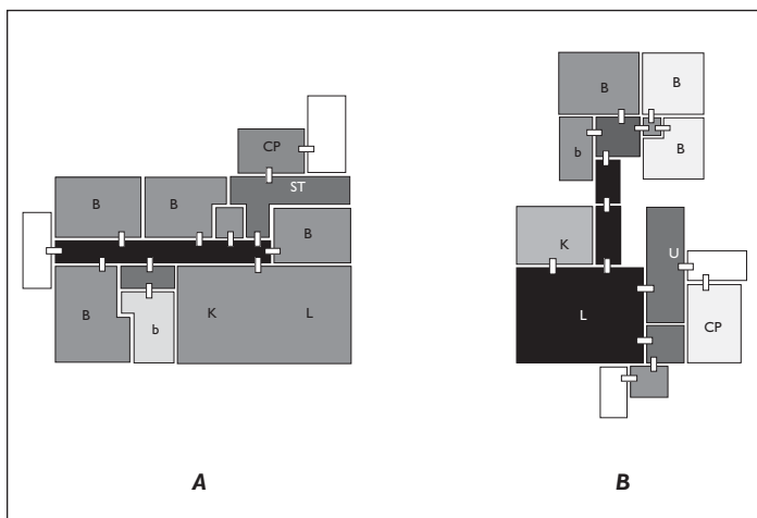
Figure 3 Processed convex breakups of an Access 4-bedroom house (A) and a Coldstream 3-bedroom house (B)
