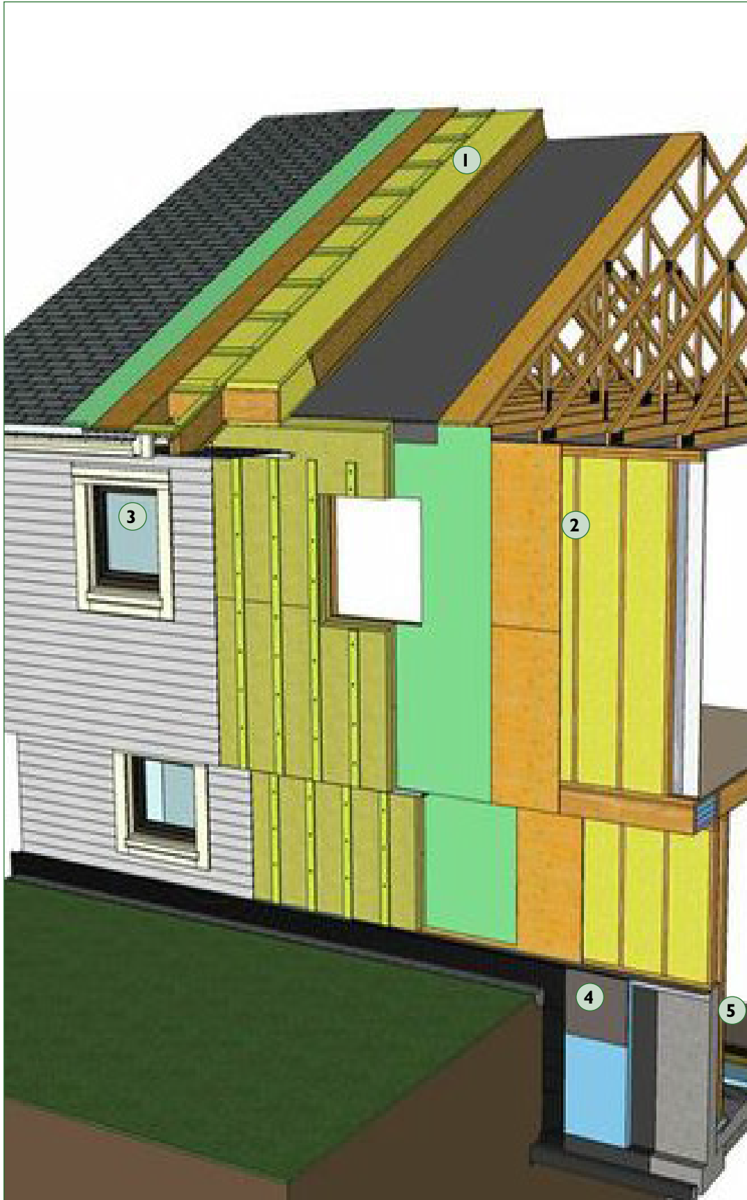
Figure 3: Post-retrofit section through roof and ceiling, above and below grade walls, floors and basement slab of a raised bungalow.
