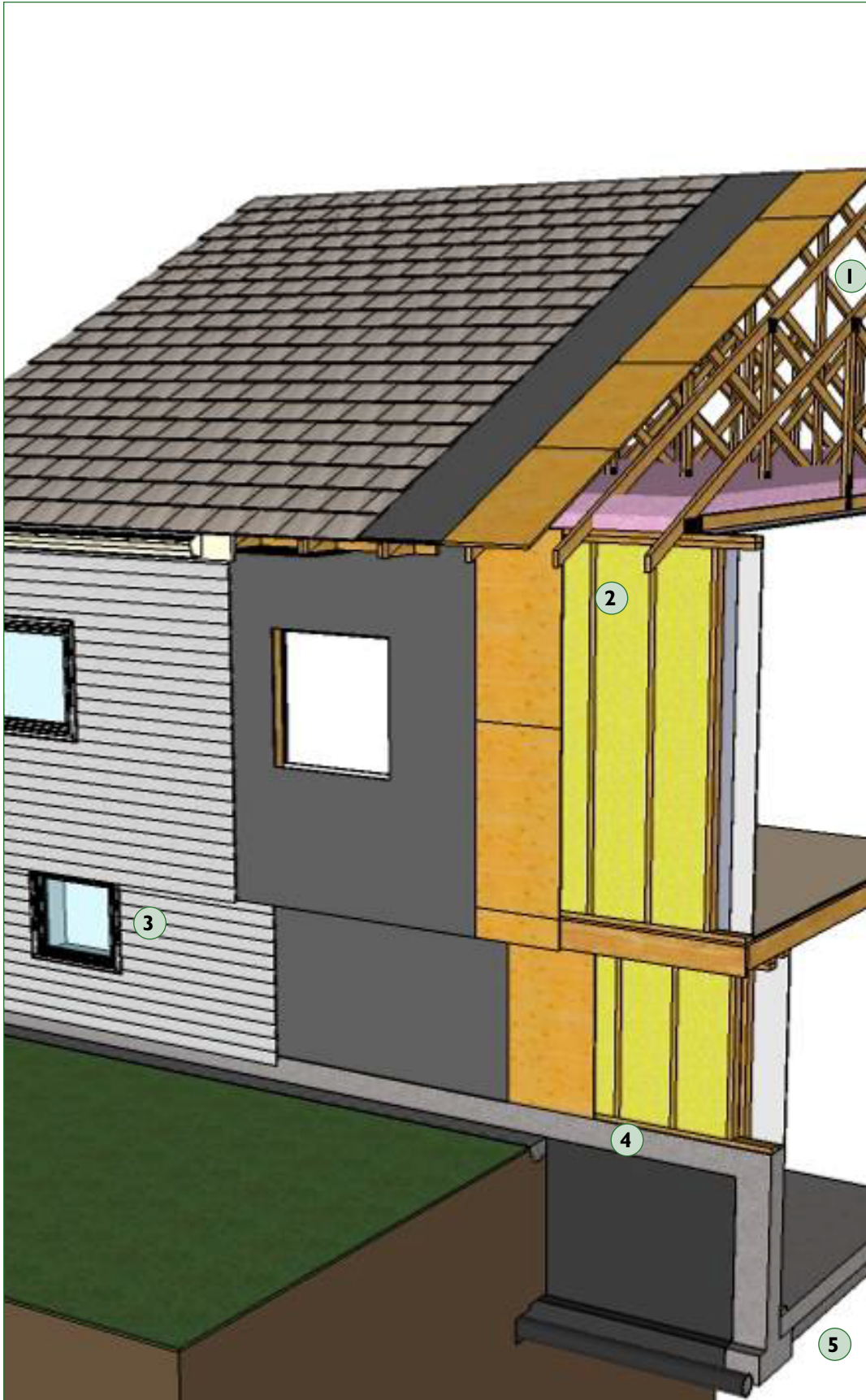
Figure 2: Pre-retrofit section through roof and ceiling, above and below grade walls, floors and basement slab of a raised bungalow
